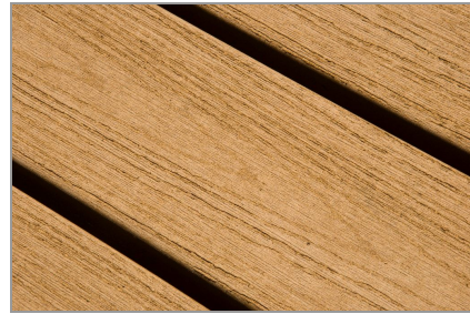
This looks like wood, but it's actually a composite of natural fibers and plastic.
